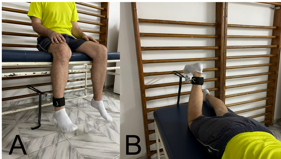
Figure 1. Participant position and dynamometer fixation for knee extension (A) and knee flexion (B) strength measurements.
