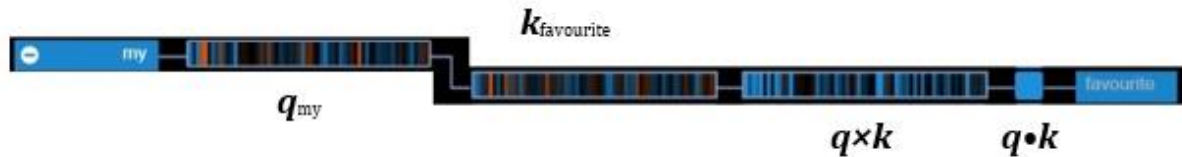
Figure 5.15: Elementwise and dot products of query ( q ) and key ( k ) vectors for next word attentions at layer 2, head 0.
