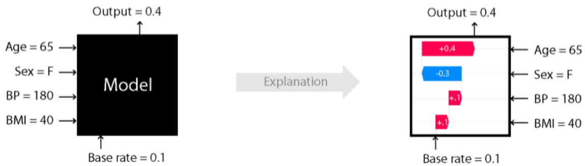
Figure 2.30: SHAP local explanation based on assigning a numeric measure of credit (marginal contribution) to each input feature [64].
