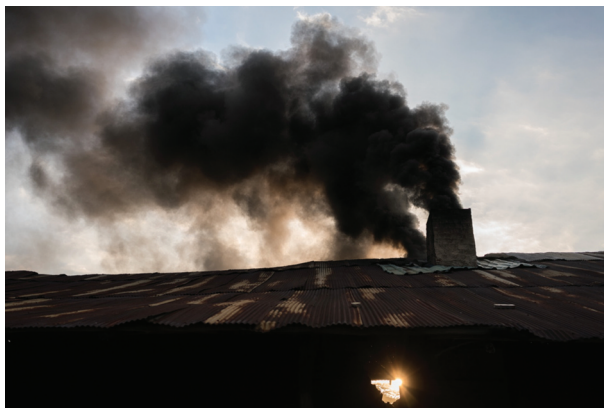
Figure 2. Black smoke emitted from a garment-fuelled brick kiln in Cambodia (Photo by Thomas Cristofolletti; copyright RHUL).
