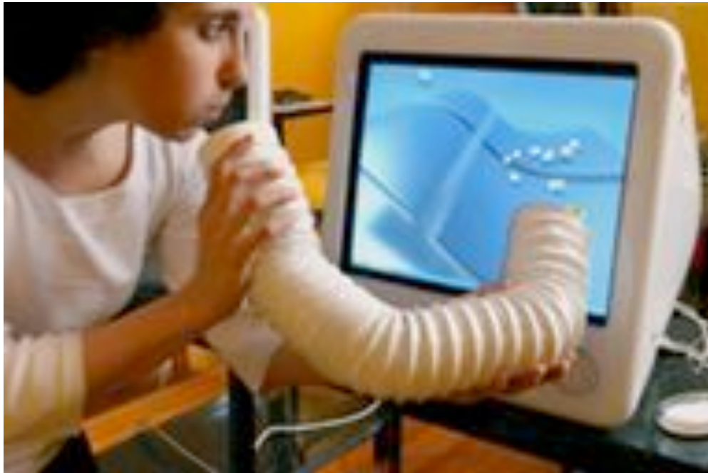
Figure 56: A user blowing into a hose to rearrange desktop icons in Blowing "Windows" [Matsumura, 2005].
