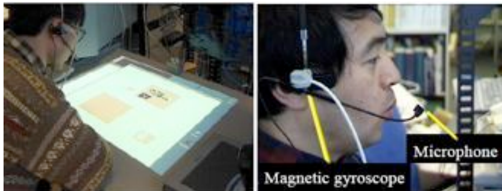
Figure 57: A user interacting with desktop objects by inhaling and exhaling into a microphone in Kirifuki [Iga and Higuchi, 2002].
