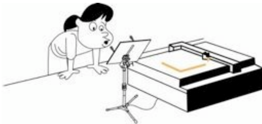
Figure 51: Blowtter : a voice-controlled plotter that allows a perhaps disabled user to blow into a mic-board in order to draw.
