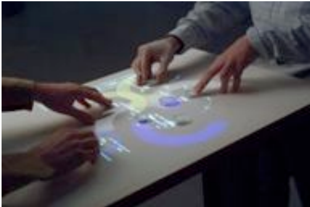
Figure 36: Audiopad ; a performance instrument that allows for live electronic music composition [Patten et al., 2002].
