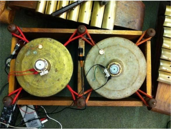
**Figure 1-4**: Iron *bonang* pots with a combination of output transducers and piezoelectric contact microphones.
