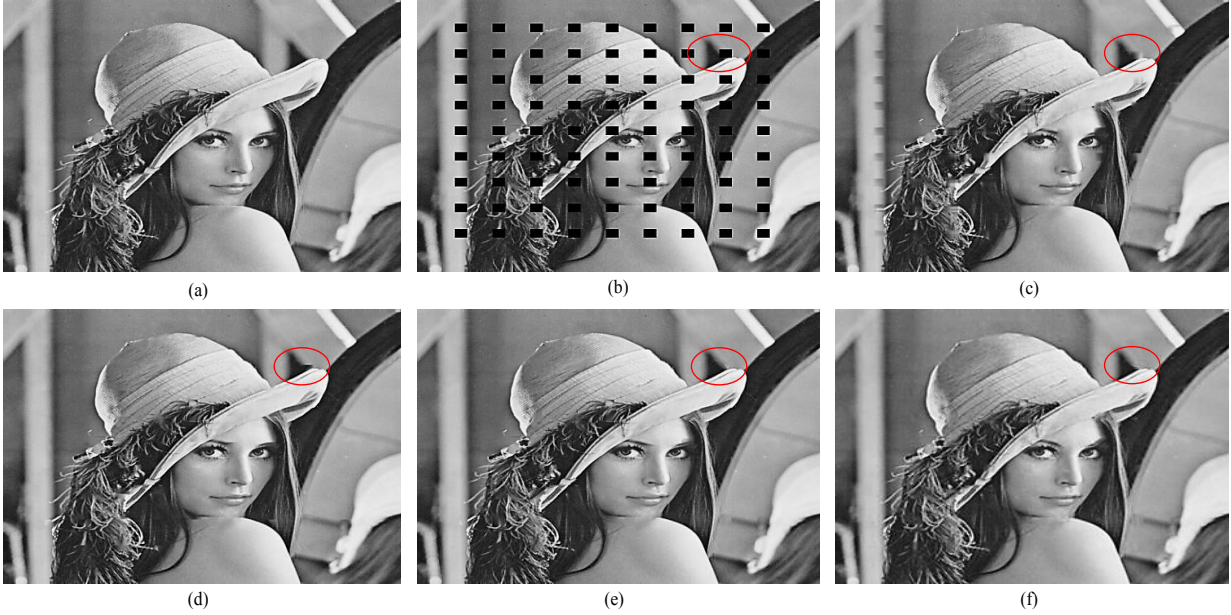
Fig. 13. Experiment on block size of 16 \times 16 pixels of the Lena image. (a) Original image 512 \times 512 , (b) damaged image blocks. Restoration using the methods of: (c) [41] (PSNR = 33.62 dB), (d) [28] (PSNR = 37.48 dB), (e) [11] (PSNR = 37.37 dB), (f) Proposed DWT (PSNR = 37.65 dB).
