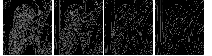
Fig. 8. Lena edge layers, from the left to right, four stages of iteration for increasing values of threshold.
