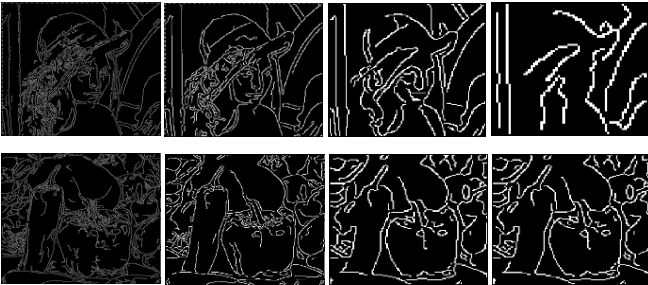
Fig. 6. Canny edge detector output for multi-scale Lena and Peppers at scales from left to right: (a) 512^2 , (b) 256^2 , (c) 128^2 , (d) 64^2 .
