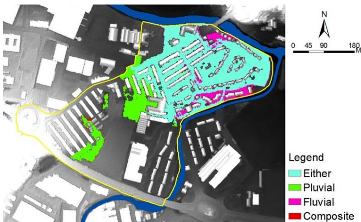
Figure 3.7: Main drivers of flooding in the Bradford case study (from Chen et al., 2010)
