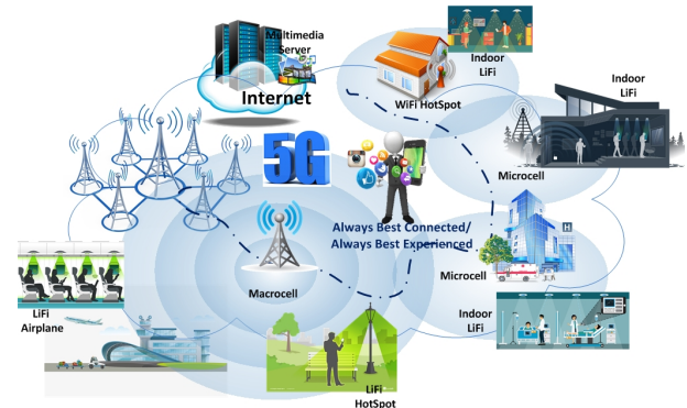
Fig. 1. Hybrid VLC/RF 5G Network Environment - Example Scenario
