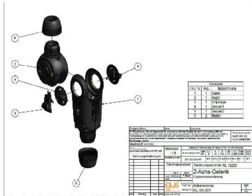
Fig. 16: Exploded drawing / parts list - 2 axes joint RL-50-001 (-002)
