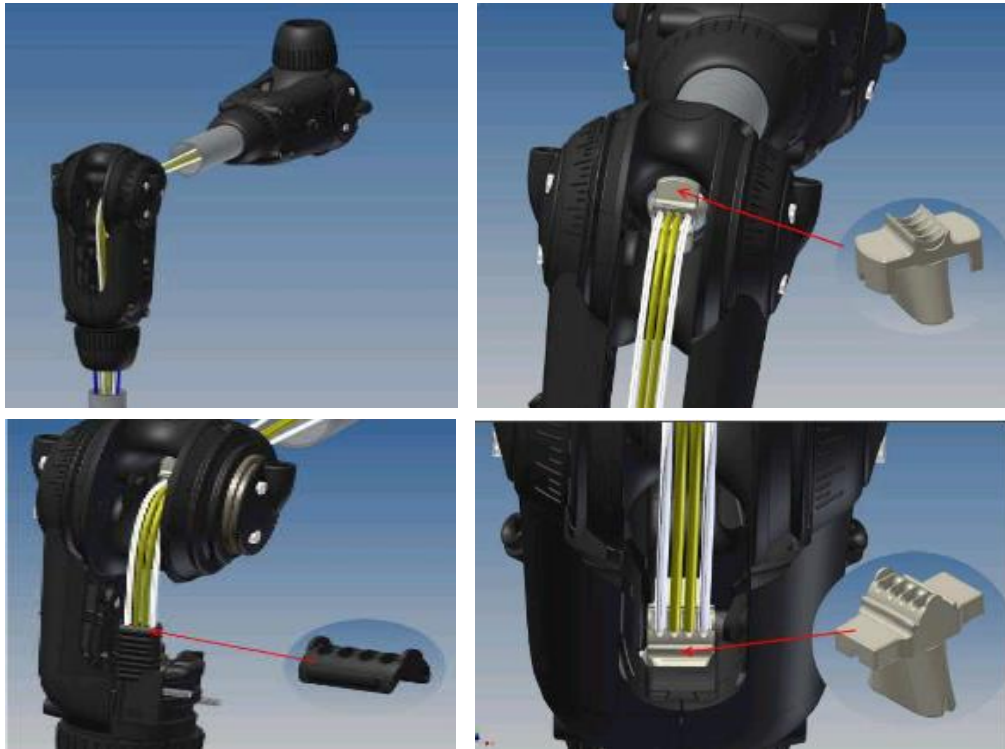
(a, b, c, d): Feeding of wires through joints (IGUS, 2012a).
