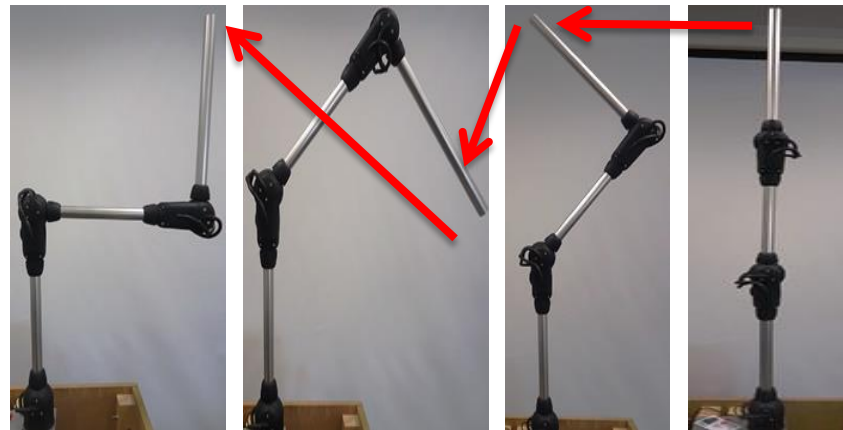
Figure5. 7: Graphical representation of point-point motion
