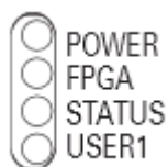
LEDs indication for cRIO 9074 (NI, 2010)
