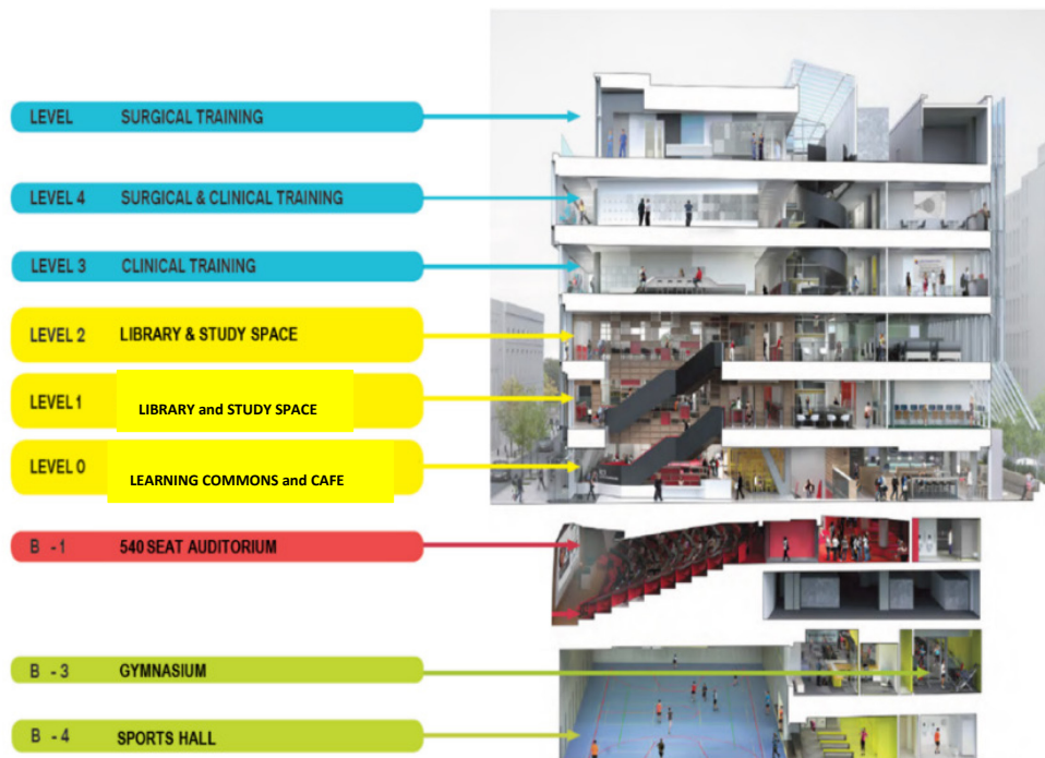
FIGURE 39 3D SECTION OF N-BUILDING WITH GUIDE
