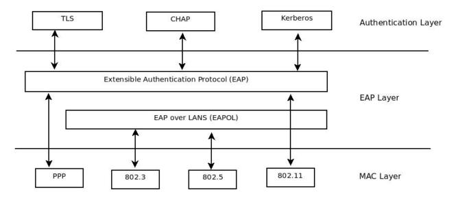
Figure 2.1: The EAP stack
