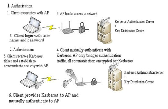
Figure 2.2: Kerberos in action in a wireless network
