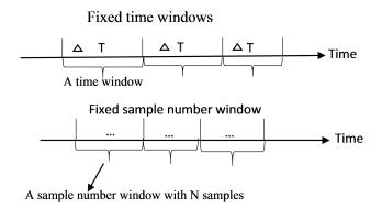
Figure 2.4: Fixed time and fixed sample number of windows for data segmentation
