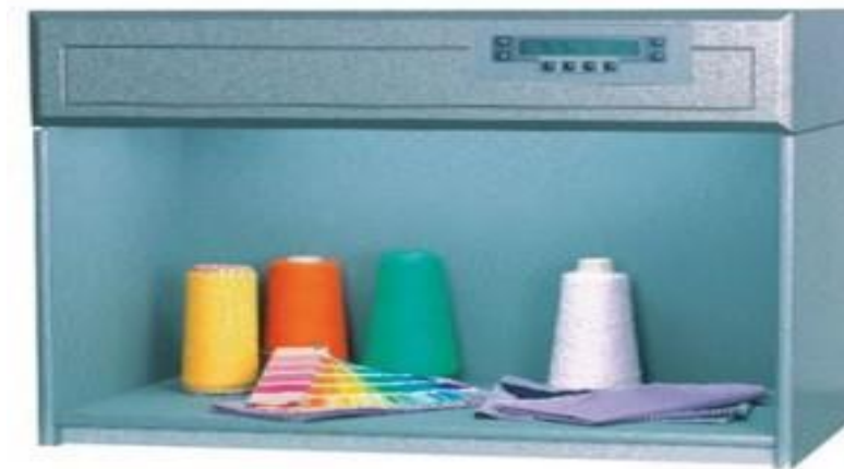
Figure 3.1: Colour viewing cabinet. [35]
