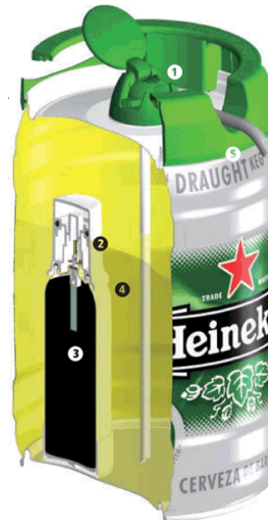
Figure 4: Cutaway showing the Heineken DraughtKeg ® system [6].
