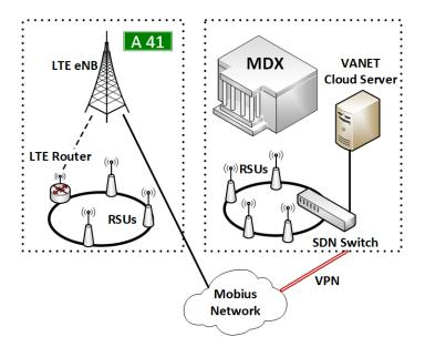
Fig. 5. MDX VANET Testbed Network Diagram
