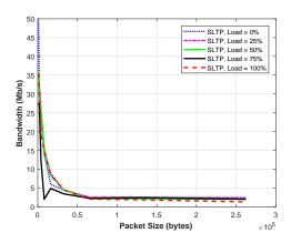
Fig. 12. RSU to RSU - Bandwidth on Load: SLTP
