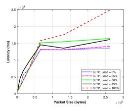
Fig. 13. RSU to RSU - Latency on Load: SLTP
