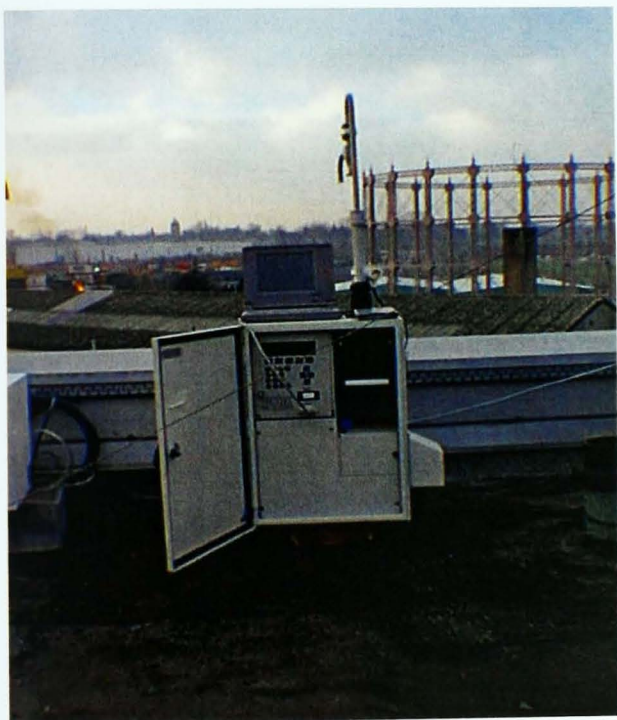
Figure 12: The Partisol 2000 'Hub' fitted with cyclonic PM_{2.5} inlet and laptop downloading stored data
