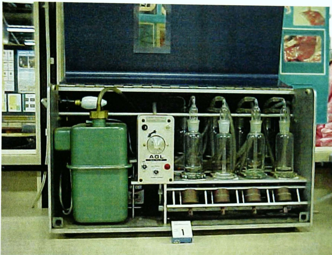
Figure 14: The black smoke sampler with side open showing gas meter, timer, bubble jars, filter clamps and a box of filters.
