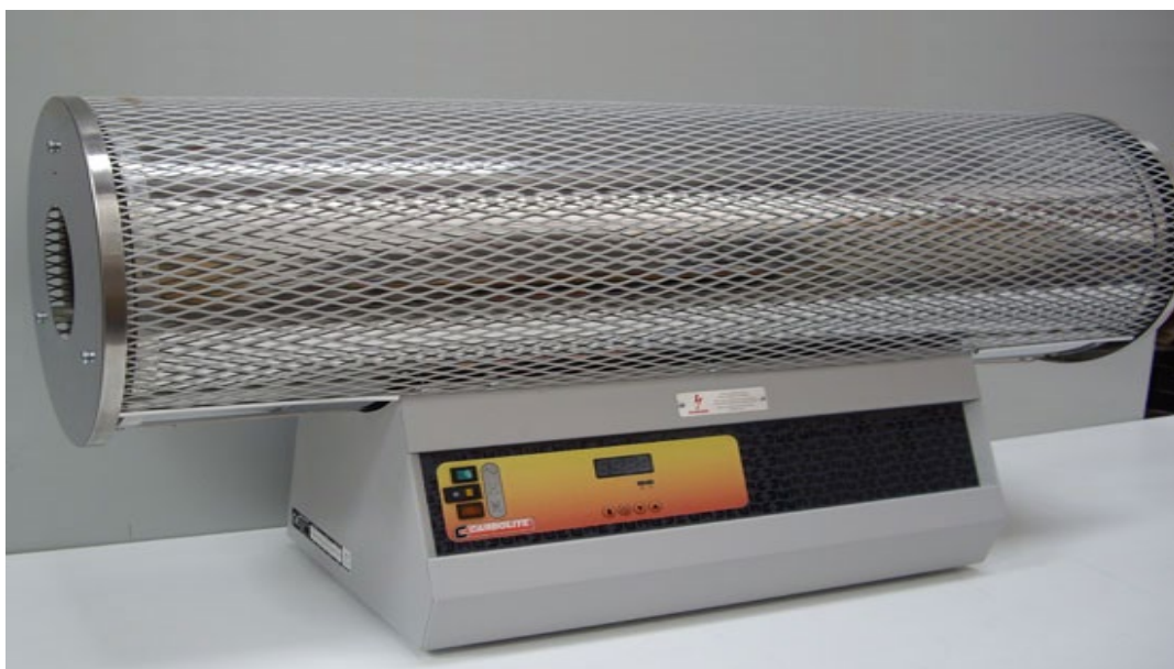
Figure 3. 4. Bench scale tube furnace at BEACON Biorefining Centre
