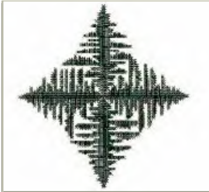
Figure 4.8: A large simulated traffic jam on a 256 \times 256 one-way grid network
