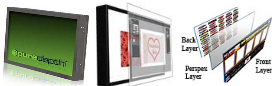
Figure 1-1. The MLD, a side-view of the MLD presenting data in each layer and a schematic representation of the MLD's layout.
