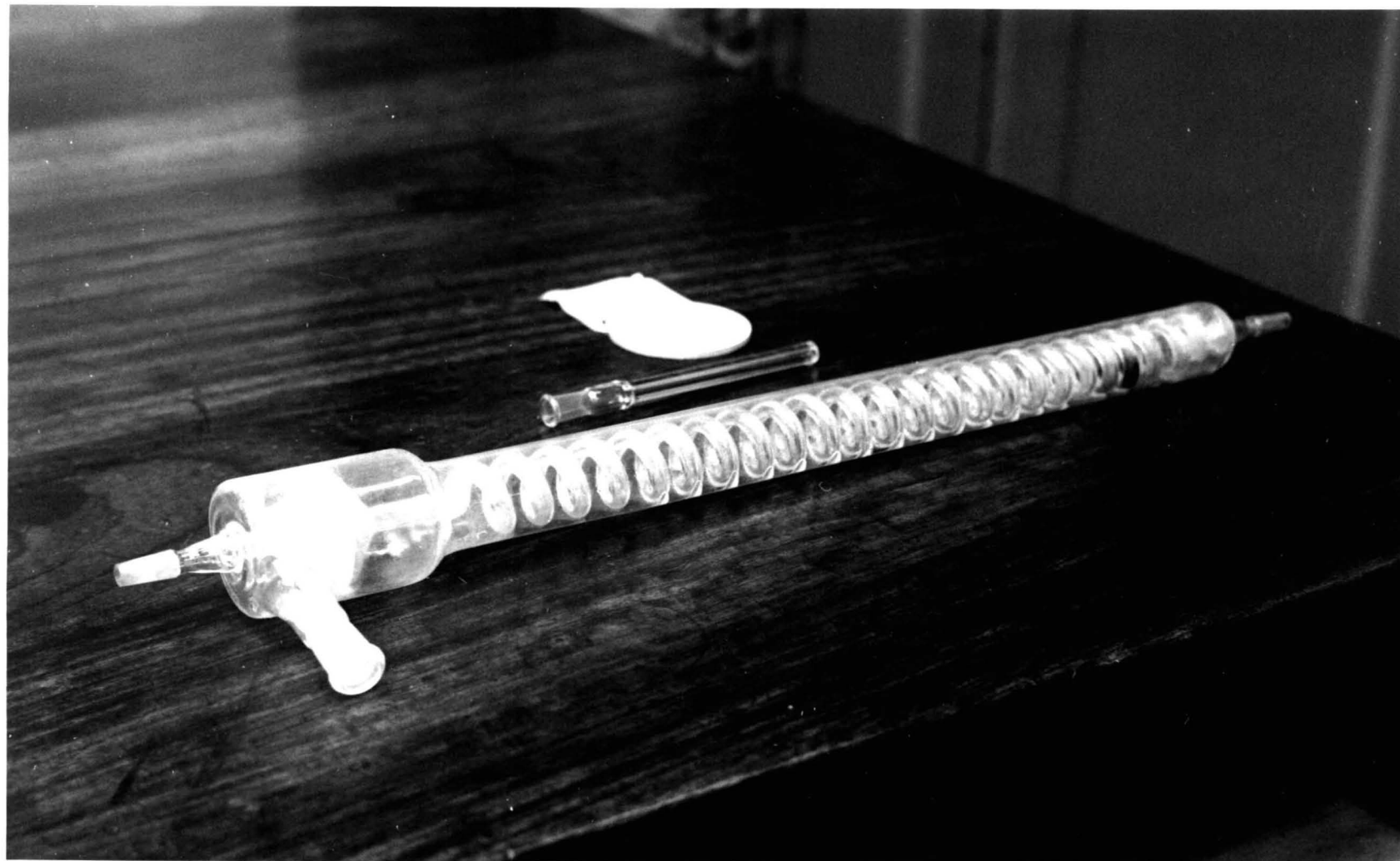
PLATE 5.1.3 General view of :- a) \text{SO}_2 collector b) Quartz sampling tube c) Stainless steel sintered disc.
