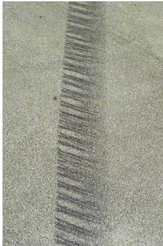
Figure 4: Striated Tyre Marks
