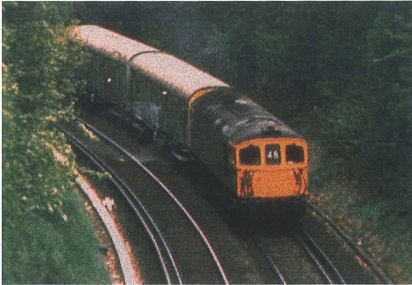
Plate 3-1 Modified rolling stock used for herbicide application to railway lines
