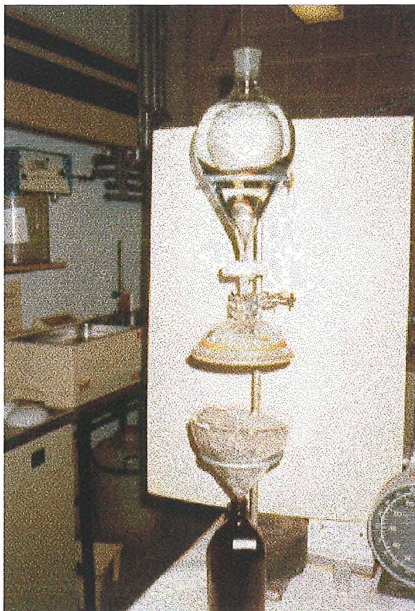
Plate 4-7 Simulated rainfall-runoff test
