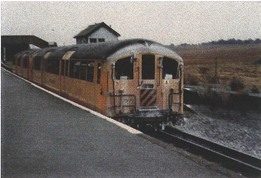
Plate 3-2 The spray train of the London Underground making a herbicide application to an above ground section of the Central Line.
