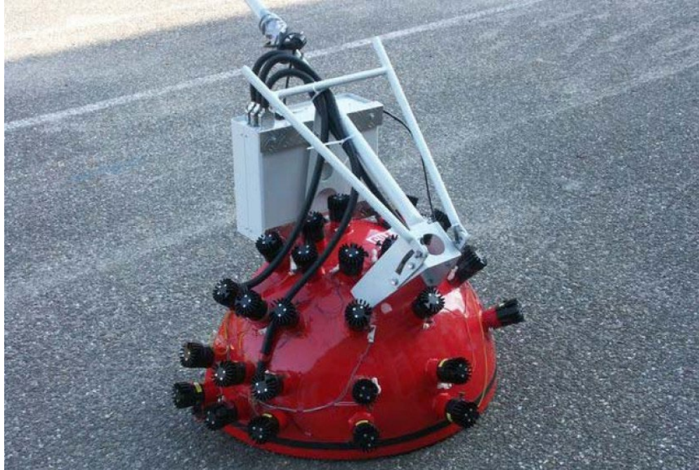
Figure 18. The Coluroute device to measure reflectivity of road surface (The Coluroute Device, 2009)
