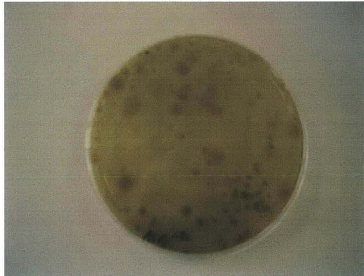
Figure 7.2 A TSA plate showing the domination by the brown colonies of bacteria isolate 1 from a MFR water sample
