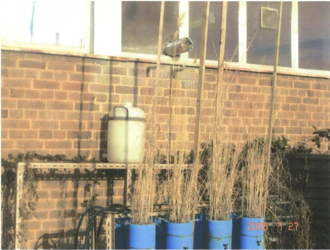
Figure 1 Section of the Pilot-Scale Vertical flow column during the winter
