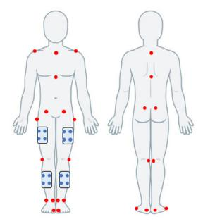
**Figure 1.** Anatomical body land marker locations of the 26 single reflective markers and four sets of non-collinear cluster markers were adhered symmetrically on both sides of each participants' body.
