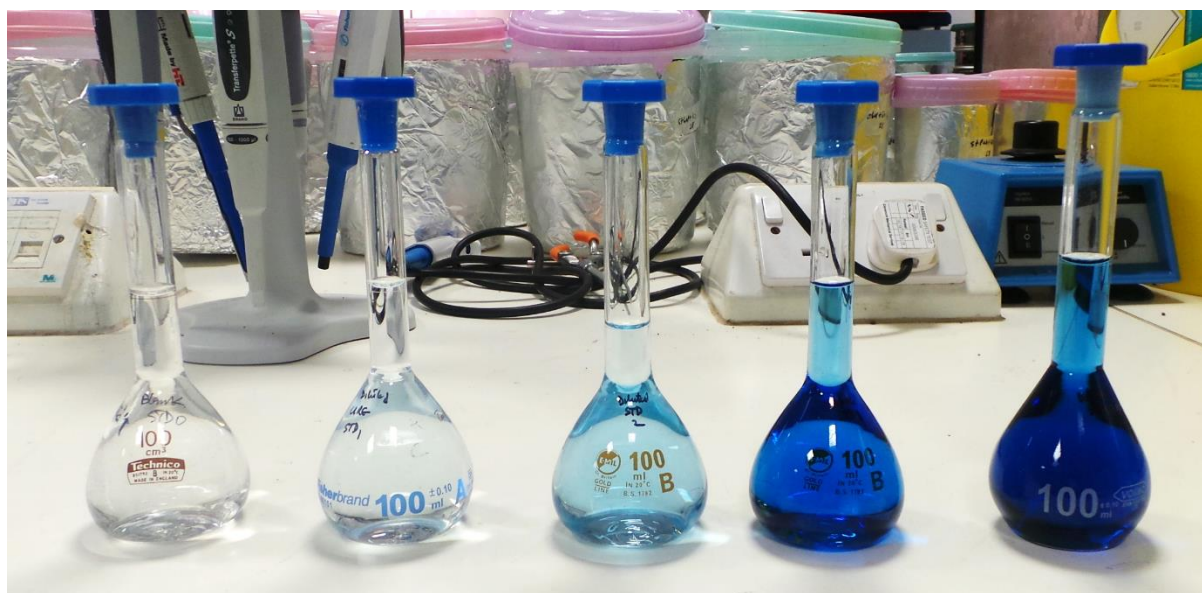
Plate 1.11 : A series of five standard solutions from Indophenol blue colour method in increasing concentration from left to right.
