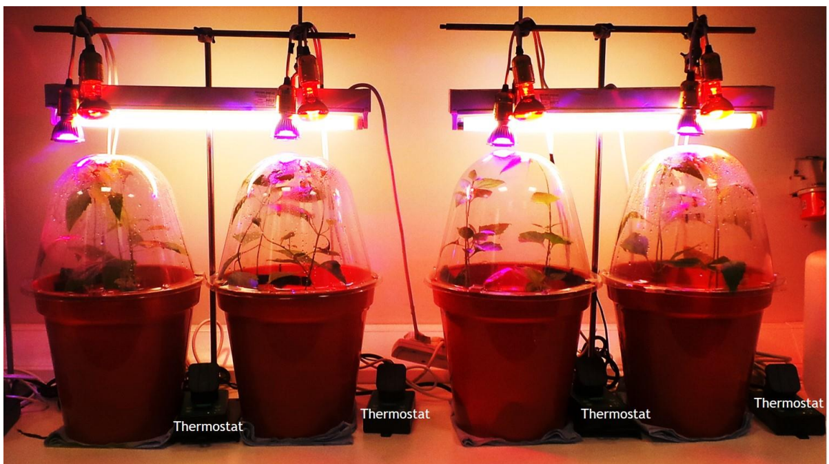
Plate 1.6(a-b): Laboratory microcosms experimental set up: (a) Solarization periods and (b) Post-solarization period (phytoremediation).
