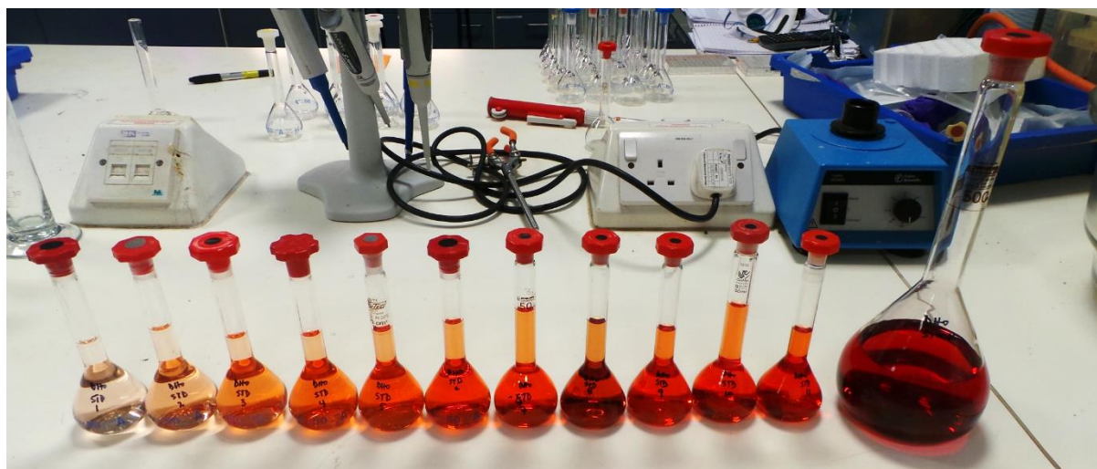
Plate 1.10 : TF solutions from stock solution in increasing concentration from left to right with the stock solution at the extreme right.
