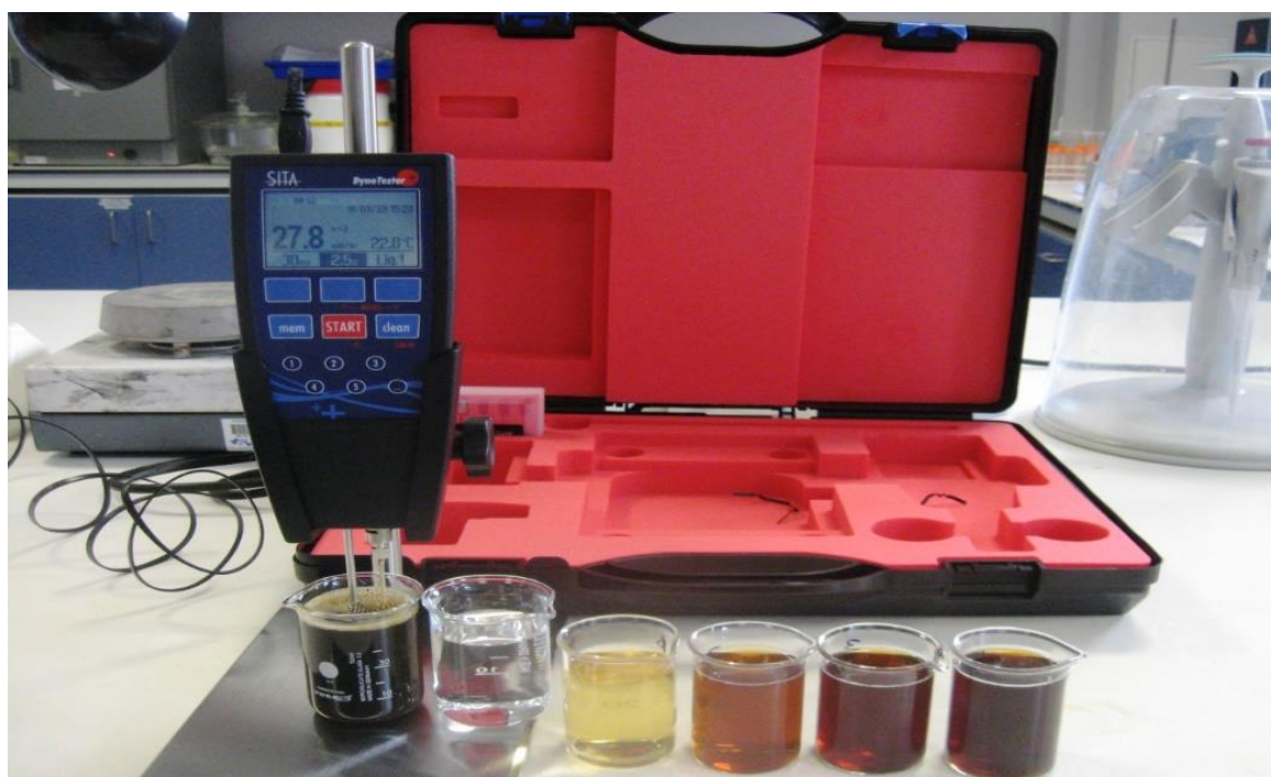
Plate 1.2: Determination of surface tension of commercial rhamnolipid biosurfactant in increasing concentration from left to right with the highest being analyzed using SITA DynoTester portable equipment.
