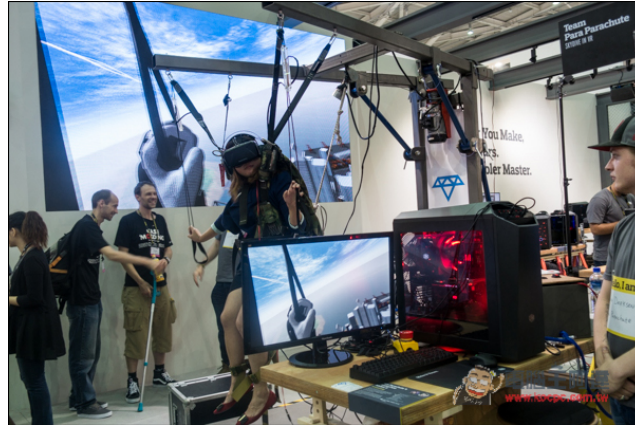
Figure 5.3: Example of a specialist virtual reality simulation involving custom user input, in this case a parachute harness allowing user movement to appear accurately virtually
