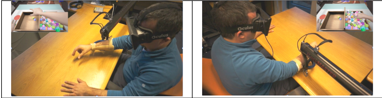
Figure 2: Able-bodied individual using the VR equipment and haptic robot system while wearing the VR glasses. Top left/right image is the virtual task (application) seen through the VR glasses (also known as Head Mounted Display).
