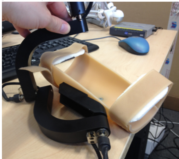
Figure 7.10: 3DOF gimbal used in the system
