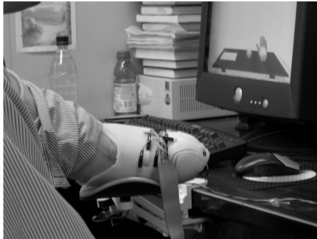
Figure 5.8: A transradial amputee participant using the system developed by Kuttuva. Extracted from [?]. Input to the virtual system is taken from EMG sensors to facilitate grasp and release with basic movement of the residual limb taken from FSR sensors.
