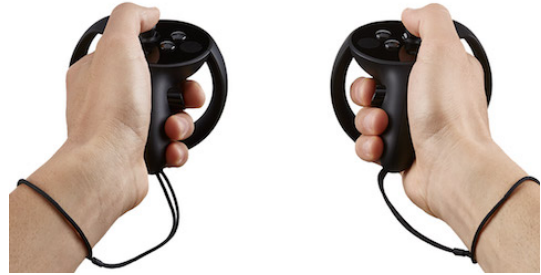
Figure 5.7: Oculus Touch controllers. For use alongside the Oculus Rift head mounted display which tracks the position and orientation of each hand as well as any button input
