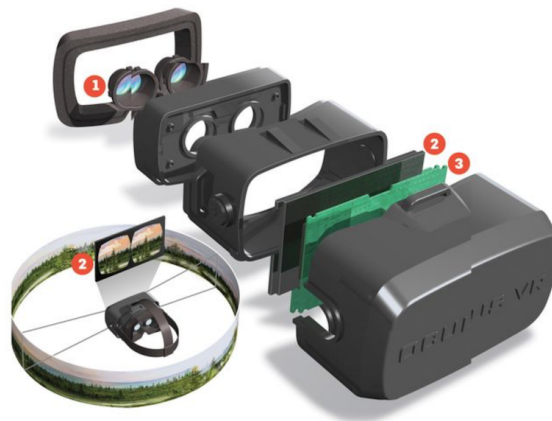
Figure D.3: Breakdown of the Oculus Rift DK2 headset with numbered parts highlighting the main components of the headset
