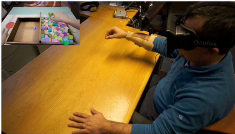
Figure 2: Able-bodied individual using the AMPSIM training system while wearing a head mounted display (HMD). Top left image is the virtual application seen through the HMD.
