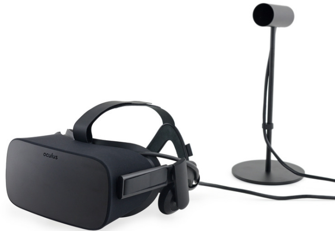
Figure D.5: The Oculus Rift CV1 with HMD tracking infra red camera
