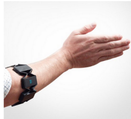
Figure 5.6: Myo, with integrated EMG sensors and gyroscope to detect arm position
