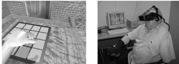
Figure 5.9: A transhumeral amputee participant using the system developed by Murray et al. Extracted from [8]. Input to the virtual system is taken from the data glove located on the intact hand mapped to the opposite amputated limb.
