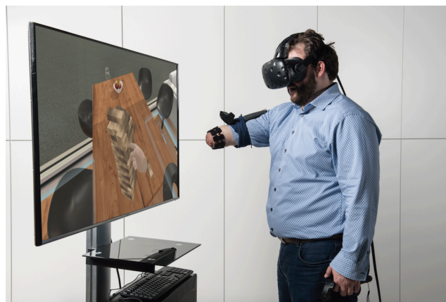
Figure 5.10: A amputee using the VITA system which uses the myo in order to achieve input to the system. Extracted from [163].
