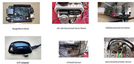
Fig. 3. Figure showing the BBB, AX-12A motors, USB2Dynamixel connector, Wifi Adapter, IR Sensor and the Gyro+Accelerometer sensor used in the experiment.
