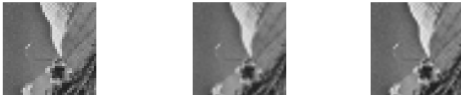
Fig. 3.12 Comparison of the three interpolation kernels. Left: Nearest-neighbour. Middle: Bilinear. Right: Bi-cubic.
