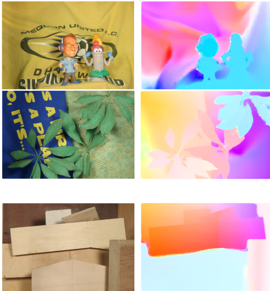
Fig. 5.13 Optical flow visualisation of some Middlebury test images obtained via steered- L^1 .
