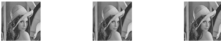
Fig. 3.13 Comparison of the three Down-scale interpolation kernels. Left: Nearest-neighbour. Middle: Bilinear. Right: Bi-cubic.
