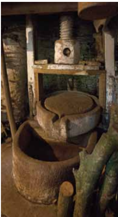
A rare example of a wooden screw cider press.
