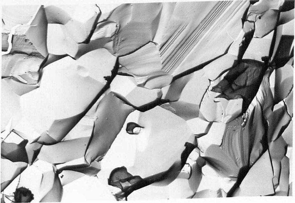
Fig.3.11.1. (g) Line of pores.20000X. (h) Fracture surface.2500X.
