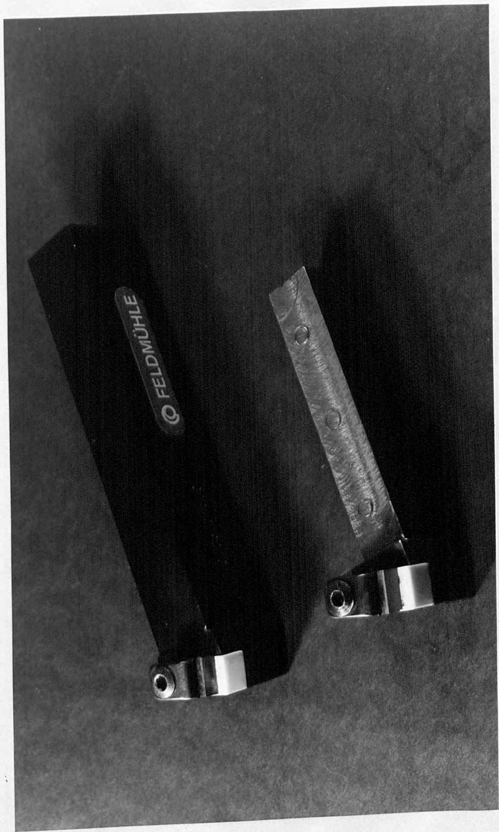
Fig.3.4.1. Duplicate tool holder reduced on shank to suit Mecalex dynamometer.
