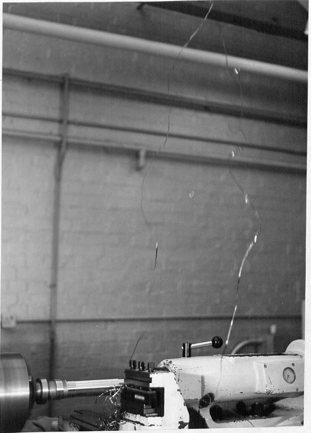
Fig.3.3.8. Swarf behaviour at cutting speed of 4500 ft/min with depth of cut 0.05 in and feed rate of 0.005 in/rev.
