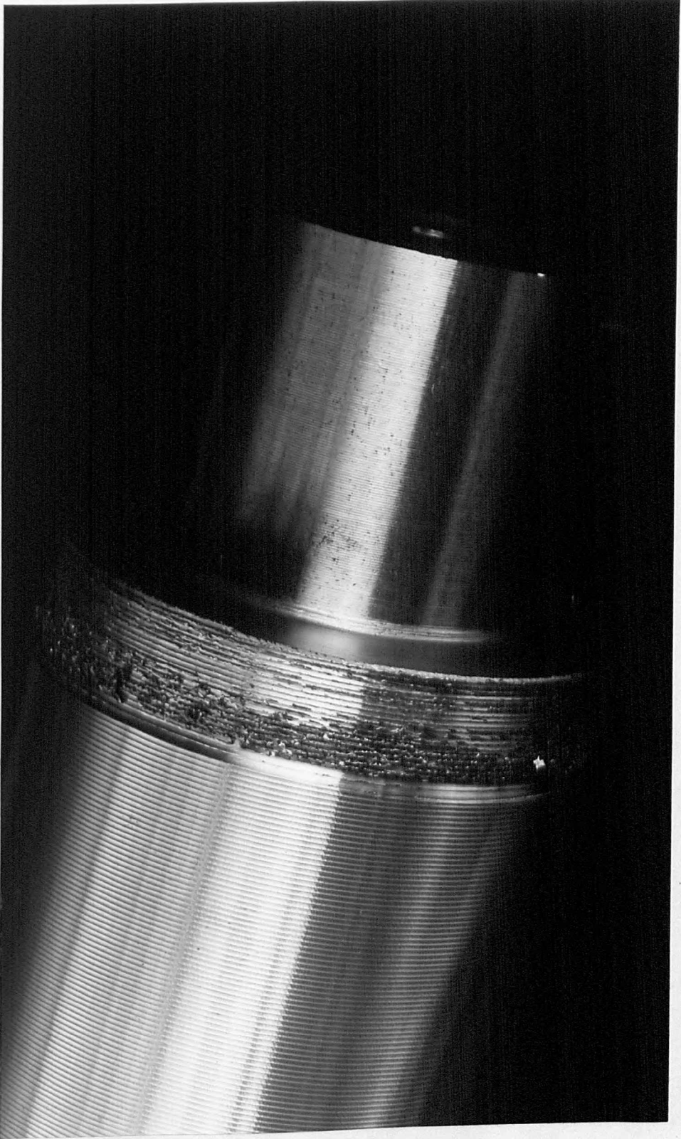
Fig.3.6.1. Illustration of re-engagement tool failure on test piece with feed rate of 0.028 in/rev at cutting speed of 1000 ft/min.
