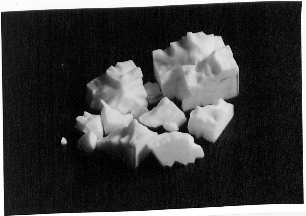
Figs.3.2.6(iii) (a) and (b). Thermal shock effects on tool tips quenched in H_2O from (a) 300^{\circ}C and (b) 700^{\circ}C .
