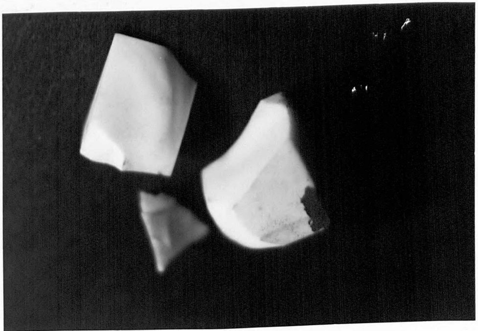
Fig.3.2.6(iv) and (v). Thermal shock effects of heating tool tip corner momentarily in (iv) a carbon arc and (v) oxy-acetylene.
