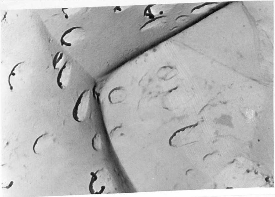
Fig.4.4(a) and (b). Showing random distribution of type 3 pore. (a) in transgranular fracture surface.13000X. (b) at grain boundaries. 10000X.
