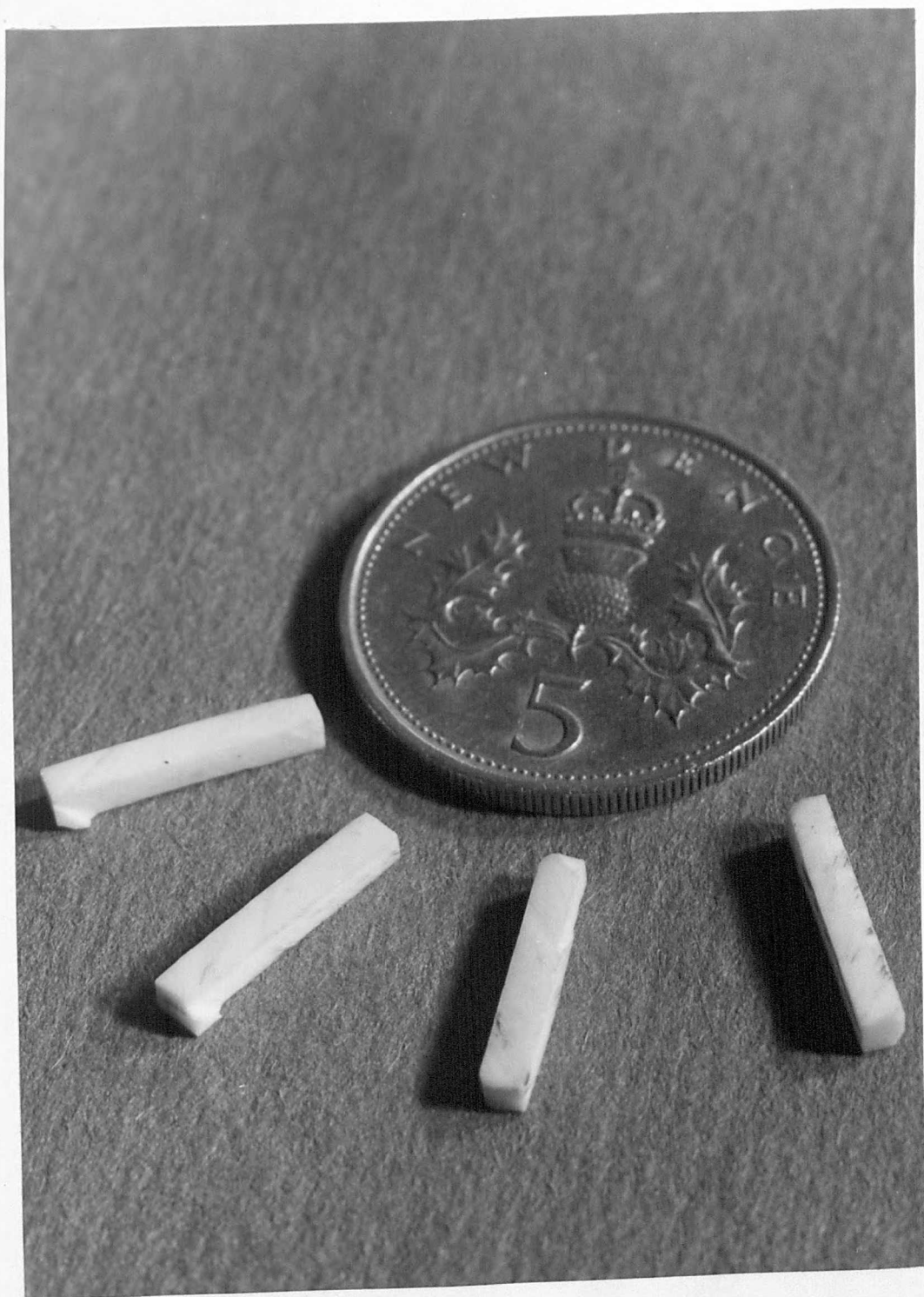
Fig.2.3.3(a). Alumina Prisms. Cut from tool tips for stiffness tests.
