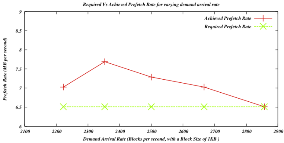
Figure 6.5: Required Prefetch Rate (6 MB per second) vs Achieved Prefetch Rate having different demand arrival rate.
