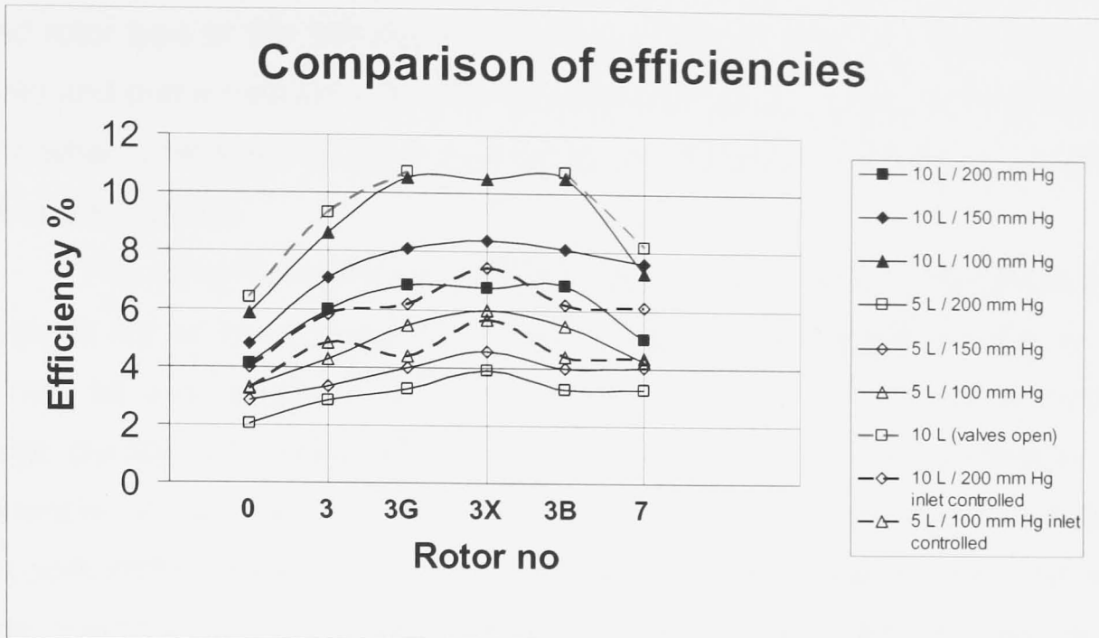
Figure 5.21. Relationship between all the rotor types and efficiency at the 'set points' for all the test fluids used.
