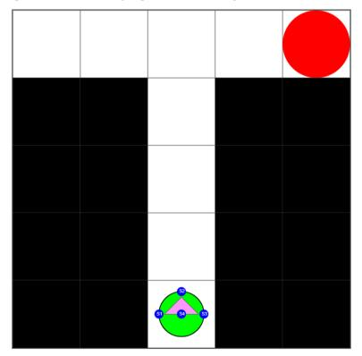
Fig. 2. Agent in maze environment. Sensors S1-S3 give the agent information about the contents of the adjacent square (empty, wall, reward). S4 gives information about the contents of the current square. The agent can rotate left and right and it can move forward into empty squares or into squares containing a reward.
