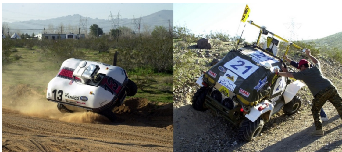
Figure 1.9 – DARPA Grand Challenge UGVs getting stuck in rough terrain. Autonomous vehicles get into trouble due to a lack of real-time information regarding ground conditions (DARPA 2014).
