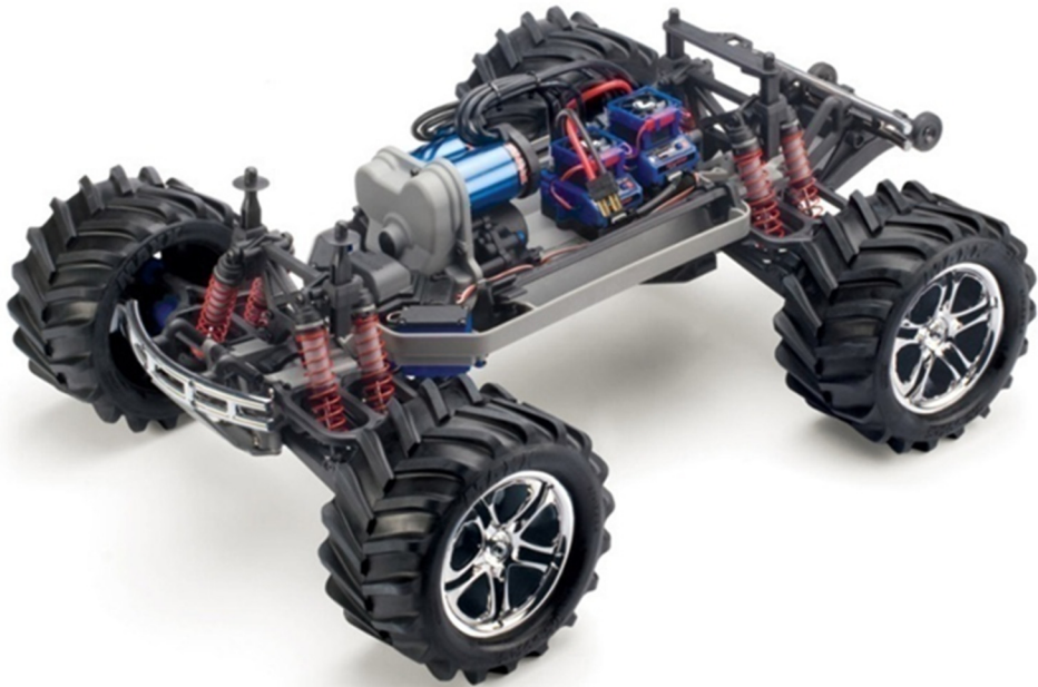
Figure 3.1 – The TRAXXAS E-Maxx off-road vehicle. This highly capable platform has been selected for the initial terrain interaction experiment (TRAXXAS 2014).
