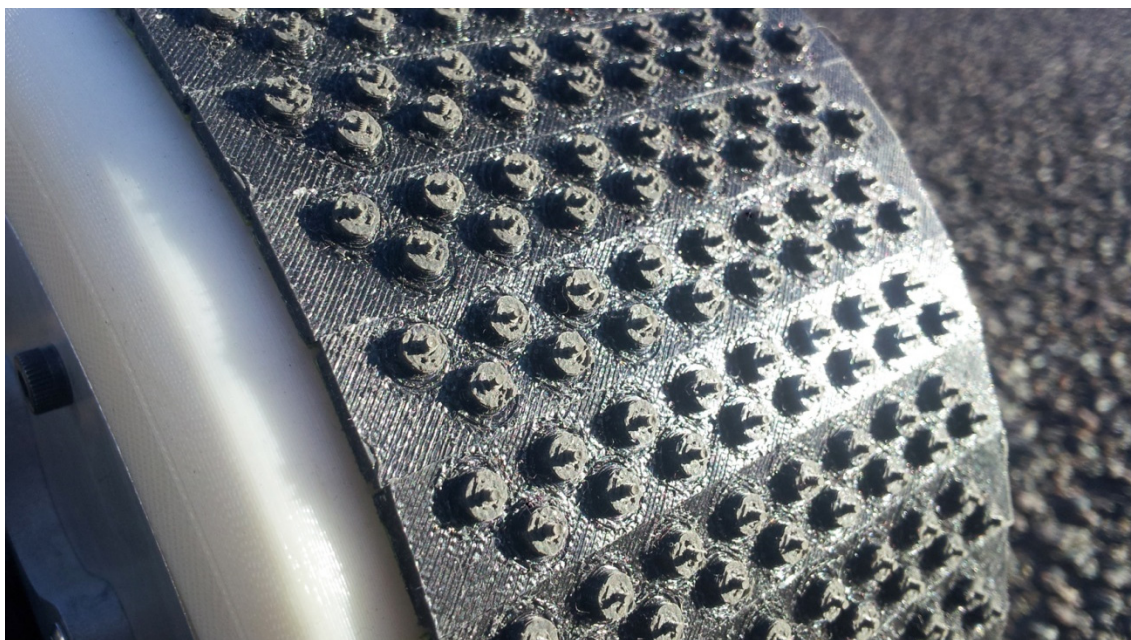
Figure 6.33 – Sensor Unit tread. The raised rubber tread helps depress the carbon pills situated below.
