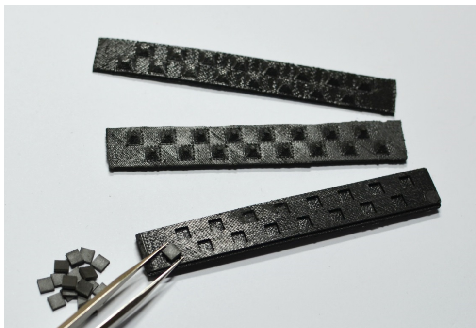
Figure 6.28 – Developed QTC sensor casing. The design of the protective casing was modified to include peaks to focus applied force onto the QTC sensors situated below.
