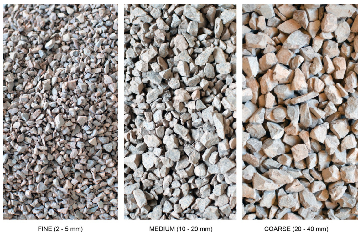
Figure 7.1 – Three grades of Gravel used for the experiment. Fine, medium and coarse gravel types were chosen as per ISO 14688-1 with the variation in grain size representing different terrain conditions.
