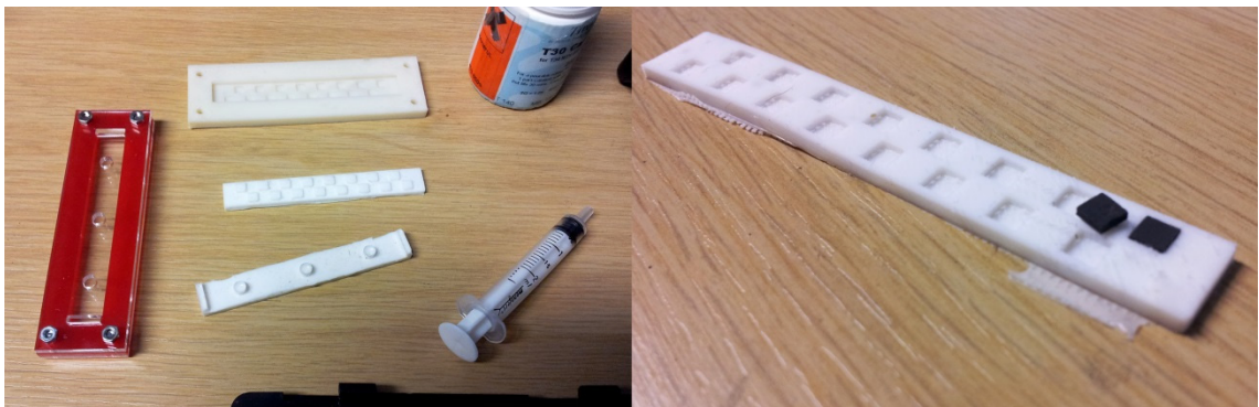
Figure 6.27 – Casting protective rubber casings. These casings were designed to protect the QTC sensors.
