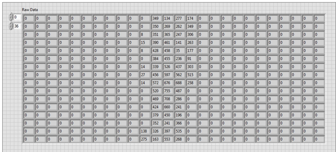
Figure 7.6 – Sensor data arranged in a 2D array. Once data packets were received from the FSW they were unpacked and arranged back into the x/y chart format using 2D arrays in LabVIEW.
