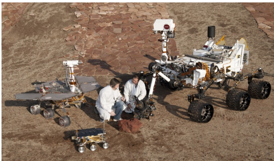
Figure 1.6 – Three generations of Mars rovers. Engineers sit with (clockwise from bottom left) Sojourner, Spirit/Opportunity and Curiosity (NASA/JPL 2012).
