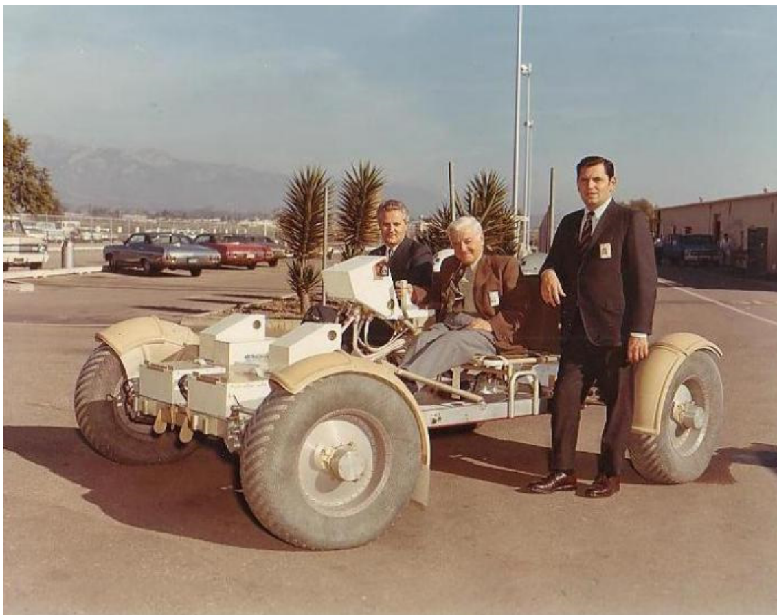
Figure 5.1 – Ferenc Pavlics, Mieczyslaw Bekker & Sam Romano with the Lunar Buggy. Dr Bekker’s pioneering work in the area of terramechanics led to the development of wire mesh tyres that could efficiently traverse the surface of the Moon (BME Omikk 2000).
