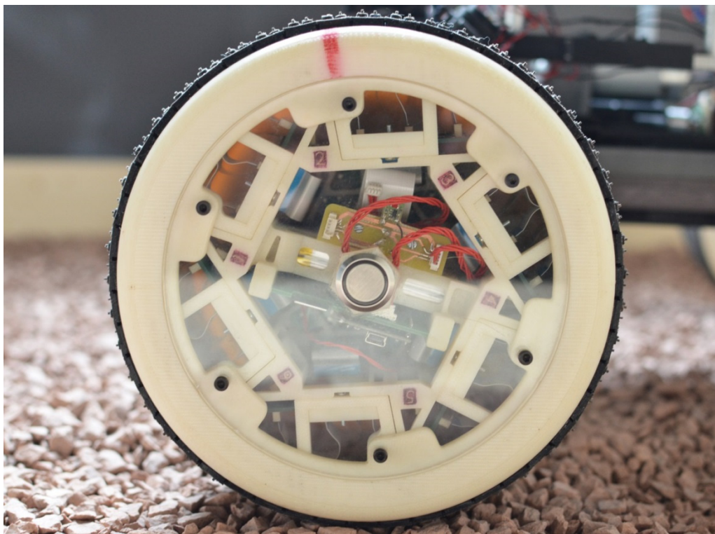
Figure 6.38 – Fully assembled Force Sensing Wheel. Once the Lock Rim was installed the Lid could be plugged in and bolted in place, completing the assembly of the FSW.
