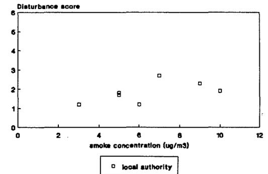
Figure 7.18 Relationship between indoor disturbance from vehicle-derived smoke, fumes and odour and median smoke concentrations (local authority data only).
