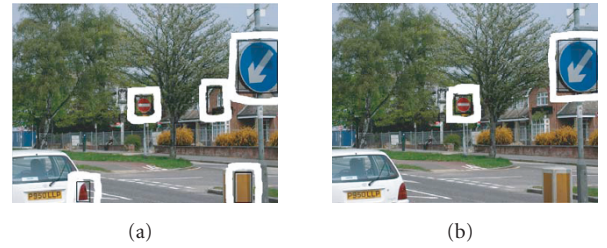
FIGURE 2: The initial results of segmentation: (a) regions marked by white contours; (b) rejection of false regions after recognition stage.
