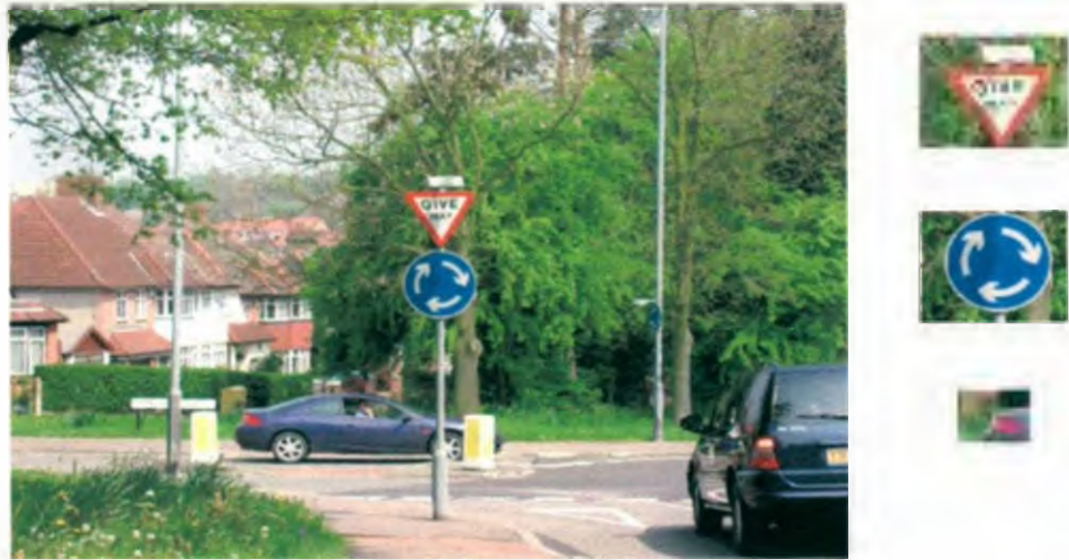
Figure 3. An example of segmented using CIECAM97 model. The third segmentation is not traffic sign that will be recognised using BMV model
