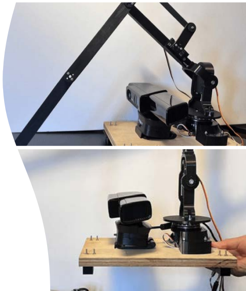
Figure 19. Compact removable standalone solution, can be attached to mobile robots for more dynamic applications
