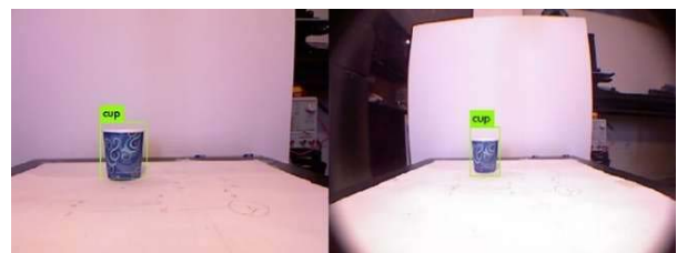
Figure 15. Zoom lens difference. The image or view of the camera without the zoom lens is much clearer and with much less distortion (left picture) than when the zoom lens is on the camera (right picture).
