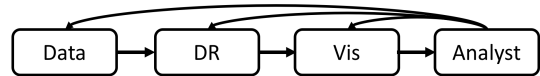
Fig. 1: A basic DR pipeline maps data to a DR algorithm. The results are visualized and presented to the analyst. Interaction feeds back to the pipeline components.
