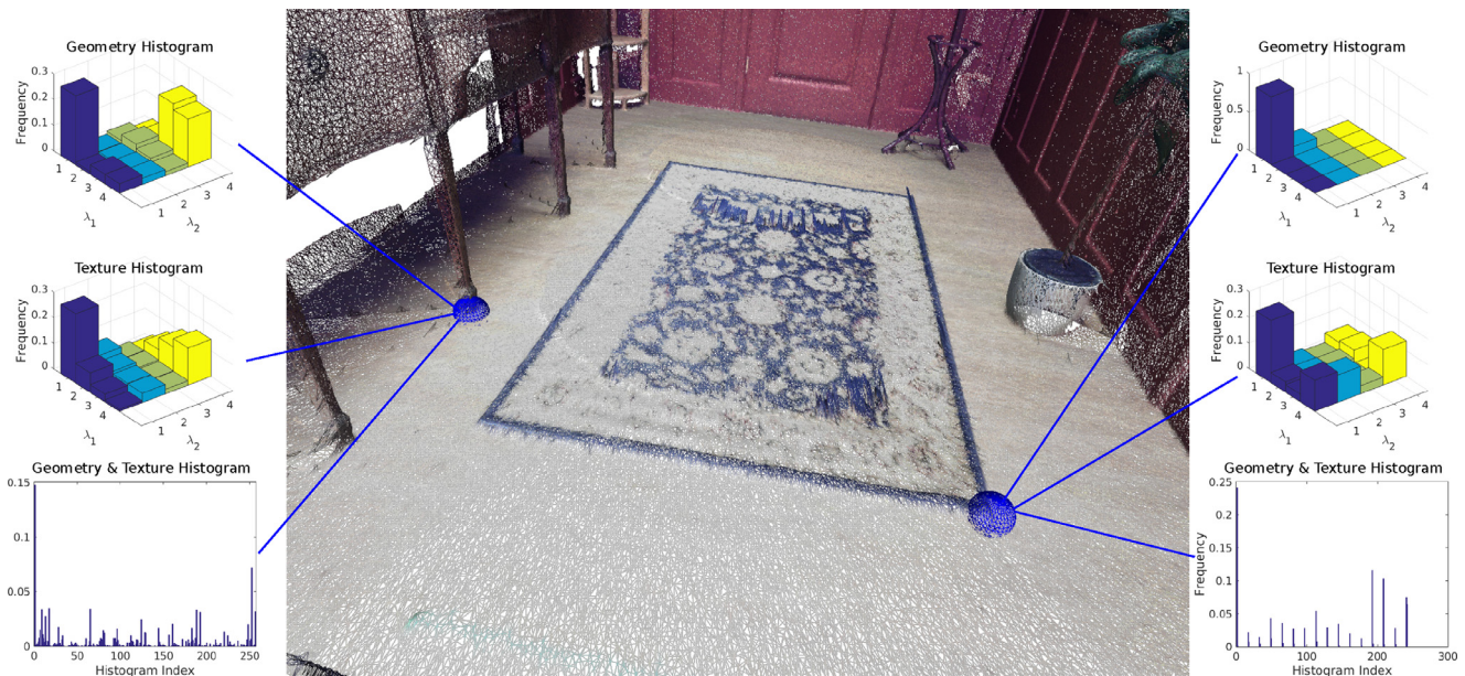
Fig. 5. An example of the derivative-based histogram distributions from 3D data when considering geometry, texture, and both. The point on the right has a large distribution of eigenvalues based on texture but not based on geometry, whereas the point on the left has a relatively larger distribution of eigenvalues based on geometry (as well as texture). In both cases, the resulting joint histogram (based on geometry and texture) is relatively sparse.
