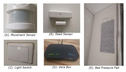
Figure 9.: Smart devices and equipment for experiments.
