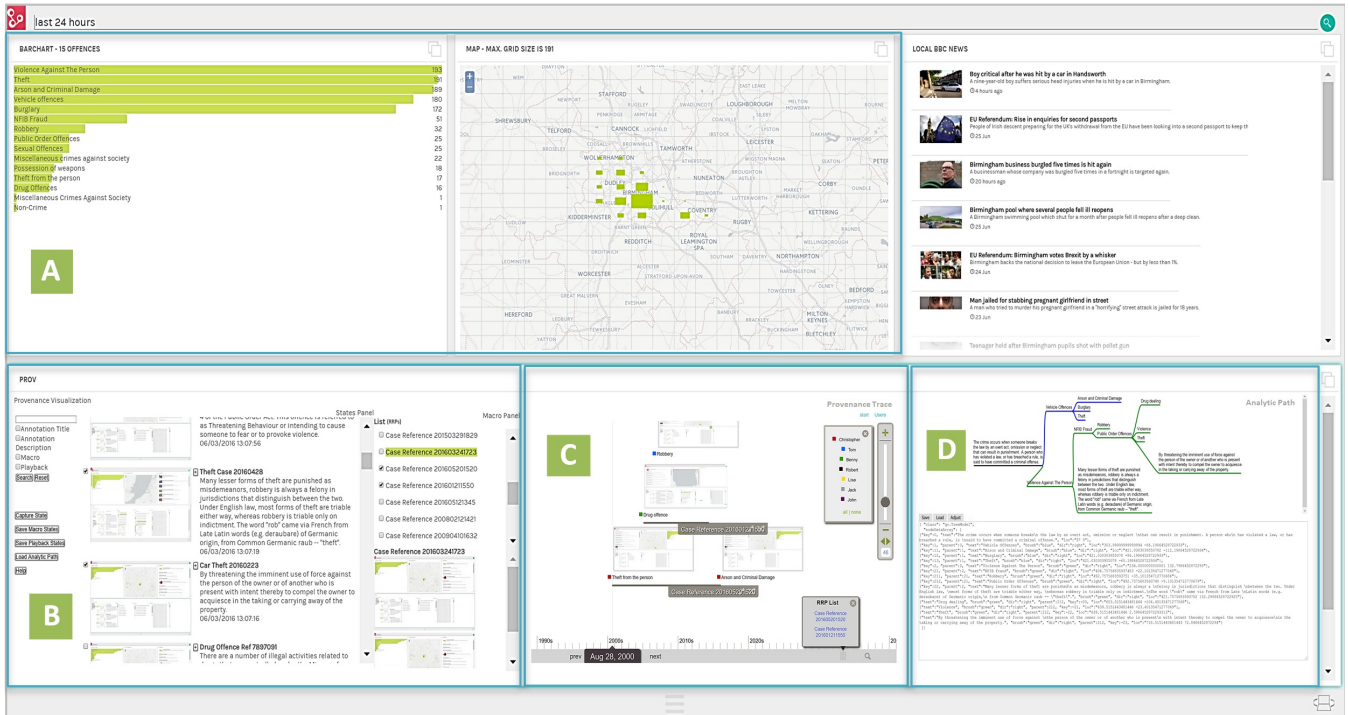
Figure 1: Four linked views for analytical provenance capture and representation system - A. Interactive partial views of AUI for total number of offences during last 24 hours on map and bar chart views, B. Captured states, macro playback panels, C. Provenance Trace panel by temporal and colour coded users (analysts) filtering, keyword search and multiple timelines selection for macro states, D. Analytic Path showing annotations set by analysts with captured states and their relationships based on interactions with colour coded users (analysts) information.
