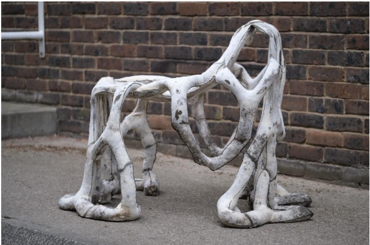
Figure 4: Example of scaled up Prototype: MycoKnit CompoSITe based on 3D knitted soft moulds.
