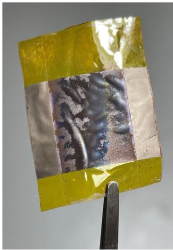
Figure 3: The TiO 2 photo-electrode prototype of dye sensitized solar cell developed on Polyimide film, which will be applied with Hogushi Ori technique in the project. (Shih, 2023).
