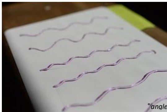
Figure 1: Outline print stroke using handheld 3d pen at 45° angle
