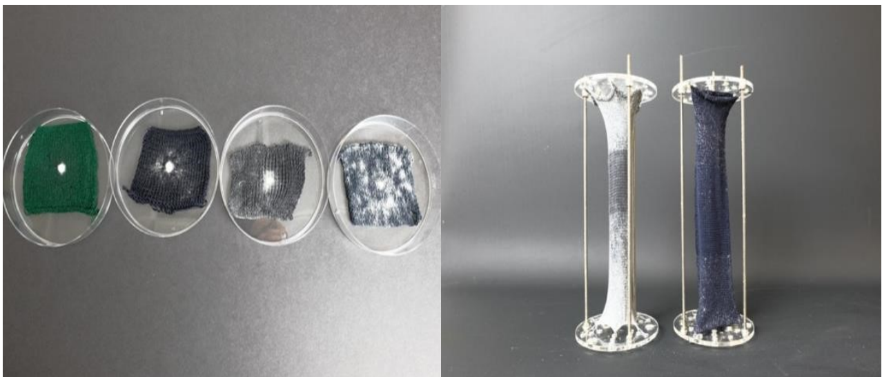
Figure 2: Experiment with knitted textiles as scaffold for Mycelium growth; various yarn qualities.
