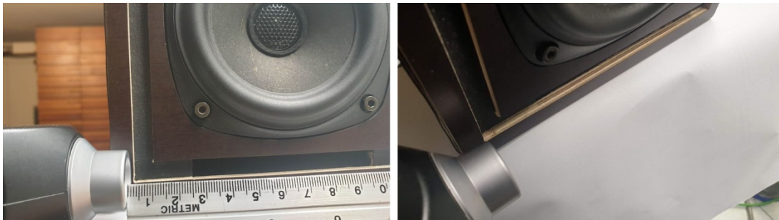
Figure G9: Measurement positions for measuring the new loudspeaker with the rectangular port.
