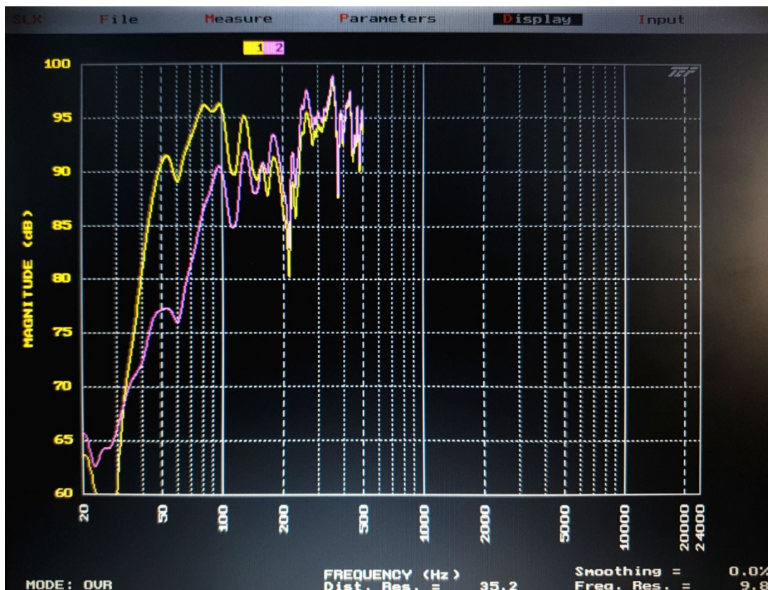
Figure 35: Bass response without (violet) and with an equaliser (yellow). Note: The comb filter on the measurement is from room reflections.
