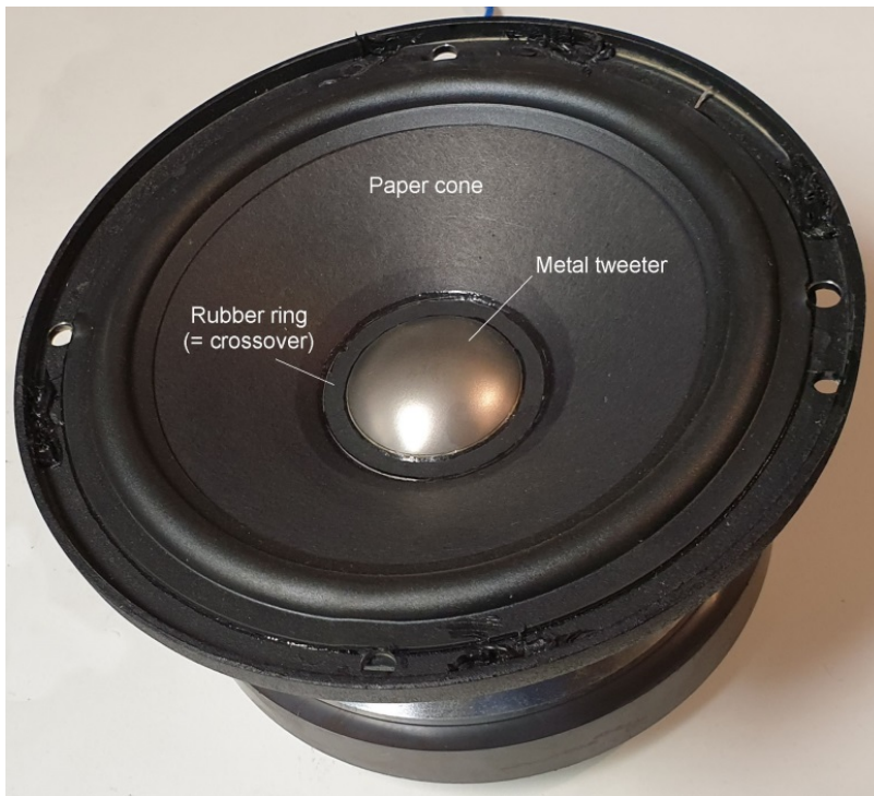
Figure 26: Two-way coaxial driver with a mechanical crossover. The rubber ring decouples the metal tweeter from the paper cone above 7kHz. Below 7kHz cone and tweeter form one large membrane.
