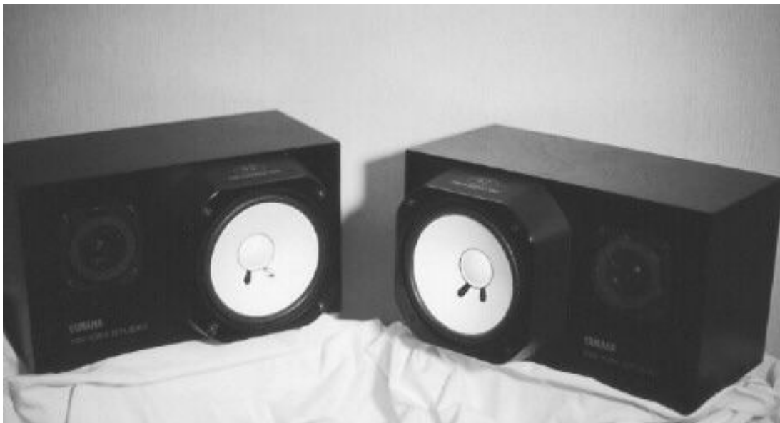
Figure 21: NS-10 loudspeakers with the Time Alignment Ring attached.
