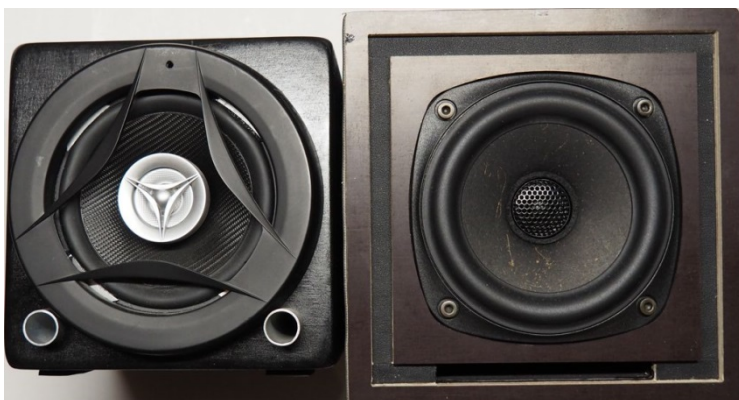
Figure 38: Original (left) and updated (right) version of the small active coaxial two-way system. Main differences are the better drivers and the longer and differently formed port.
