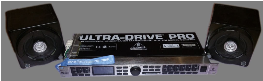
Figure 34: Small active loudspeakers with a digital crossover for demonstrating equalisation effects. On the left side of the crossover, four car hi-fi power amplifiers were integrated into the crossover.
