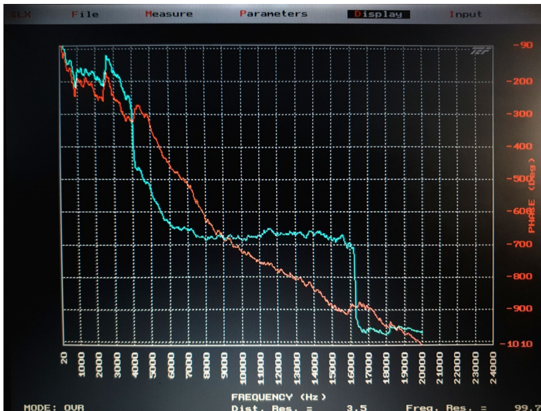
Figure 37: Phase response comparing the equalised (red) and the unequalised loudspeakers (cyan). The equalised response is getting much closer to linear phase. Note: Linear phase would be a straight line of an arbitrary angle.
