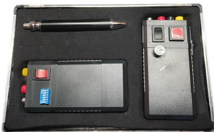
Figure 10: The author's measurement set from 1993: Top: A small Sennheiser electret microphone built into a thick pencil. Left: Mic preamp with DIP-switch-programmable gain. Right: Impulse/step-generator with trigger output.
