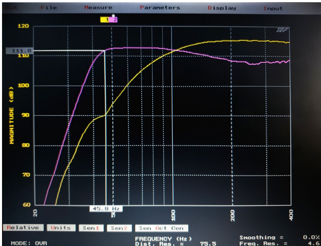
Figure G6: Frequency response of the woofer (yellow) and the port (pink) in the bass range.
