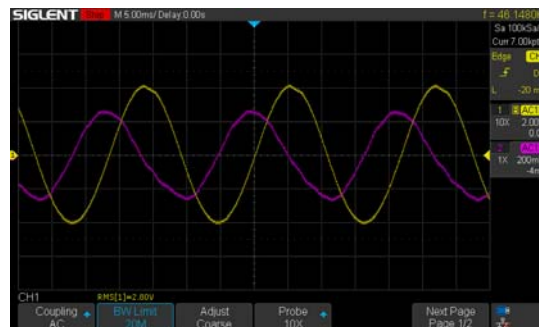
Figure G16: 46Hz/2.8V from the amplifier is applied to the woofer (yellow). The amplifier clips in the positive half-wave. The port response of the new port is shown in pink. While the output of the port still rises proportionally to the increase of the input, additional distortion is seen in the output during the period when the input signal clips.
