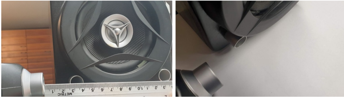
Figure G8: Measurement positions for measuring the old loudspeaker with the round ports.
