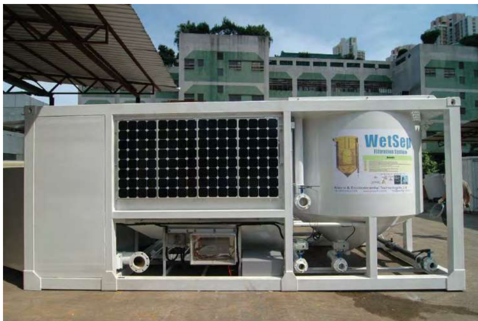
Figure 3-4 Solar WetSep filtration system.
