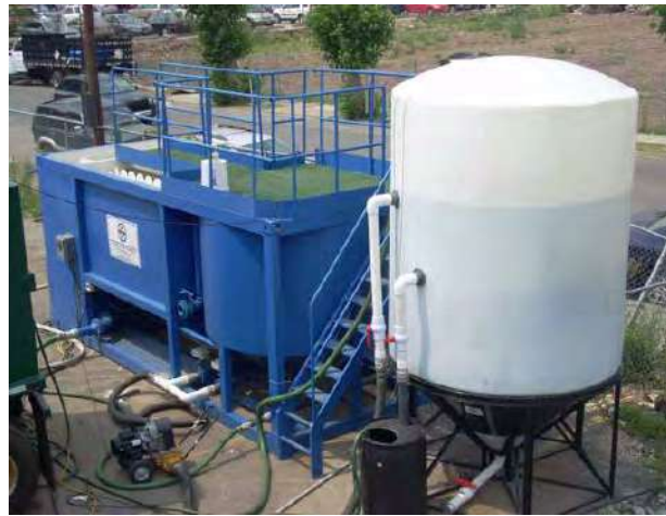
Figure 3-5 WetSep filtration system in Harrison, Middlesex Street, New Jersey, U.S.
