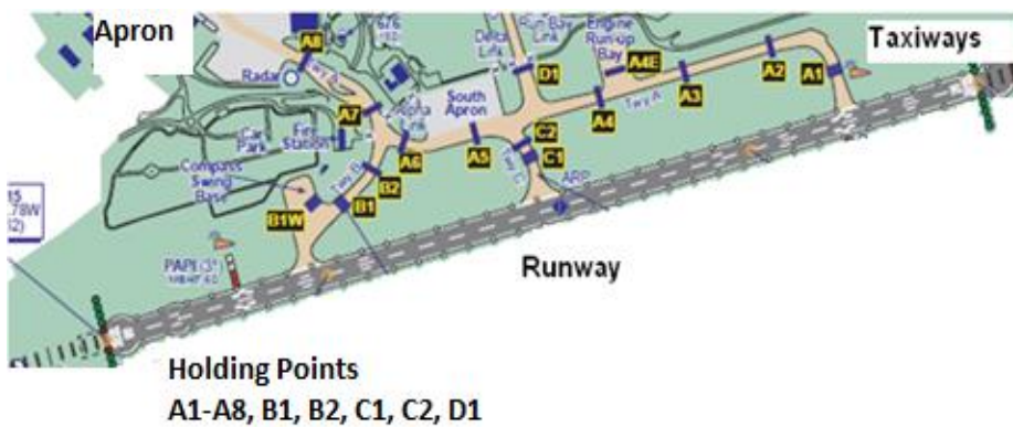
Figure 3- 3: Runway, Taxiways, Holding Points and Apron Area Layout at Studied Airport 7
