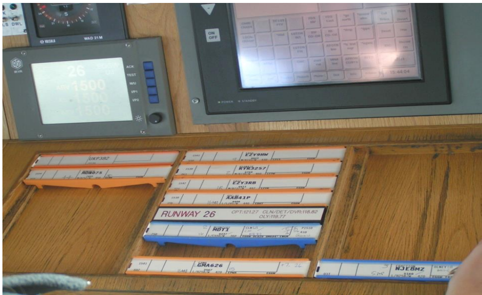
Movement of FPS on Strip Holding Bay Representing Movement of Incoming and Outgoing Aircraft
