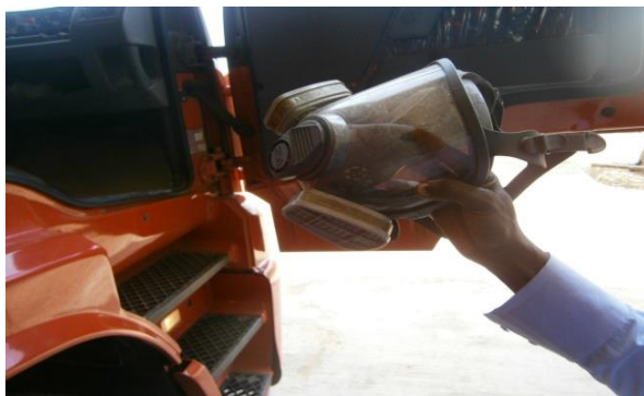
Figure 1 – A face mask used by the Nigerian firefighters in place of breathing apparatus sets
