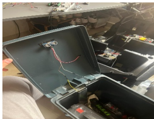
Figure 14. Ultrasonic Sensor Taped Underneath the Lid of the Trash Bin
