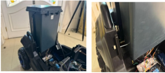
Figure 13. 35-Liter Trash Bin Mounted on Top of the Platform
