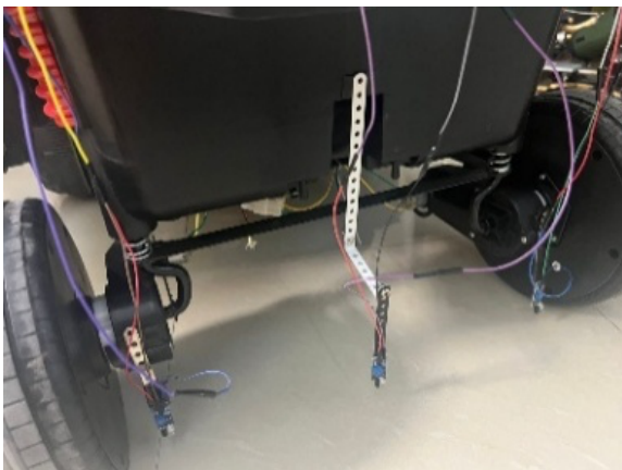
Figure 23. Three IR Sensors Attached to the Back of the Platform
