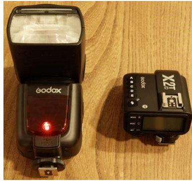
Figure 30: Speedlight with zoom head and wireless trigger
